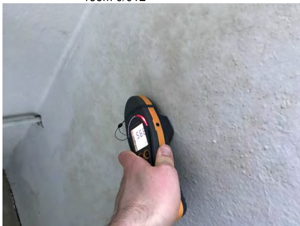
Photo 29. High moisture readings in Male Toilet
